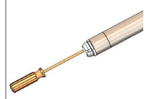
Step 9: Tighten screws until there is no gap between the Sensor Cover and the Sensor End.
