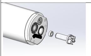
Step 6: Install new impeller and bearing for small pin impeller. For large pin impeller, replace only the impeller.
