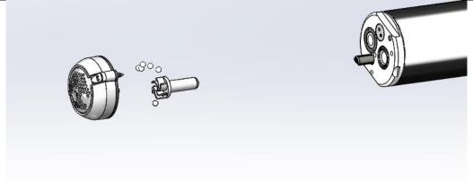
Step 3: Remove the sensor cover assembly, impeller, and cleaning beads. Note which impeller was
