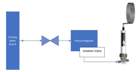
Figure 4: Tubing connection to sensor
