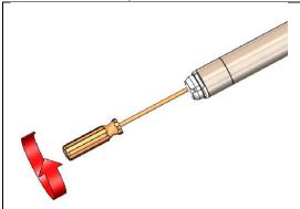
Step 1: Remove the screws holding the Sensor Cover and strainer on to the sensor end.
