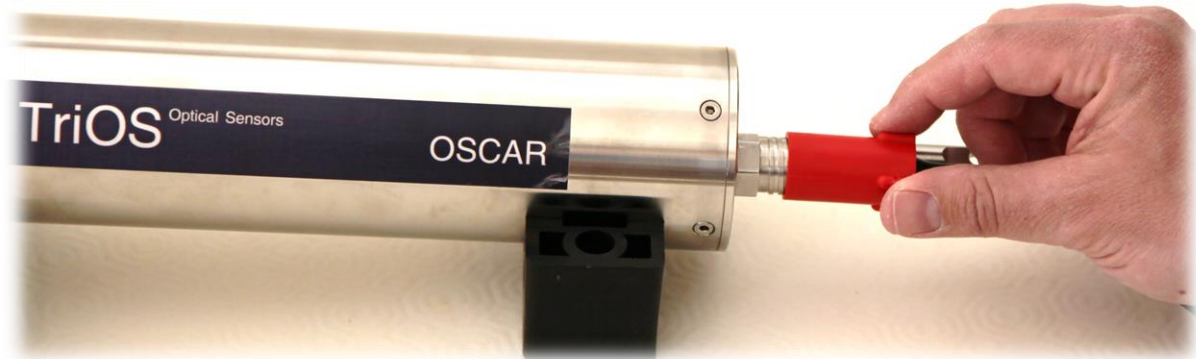
Fig. 4. Locking sleeve for fixation of the underwater connector
