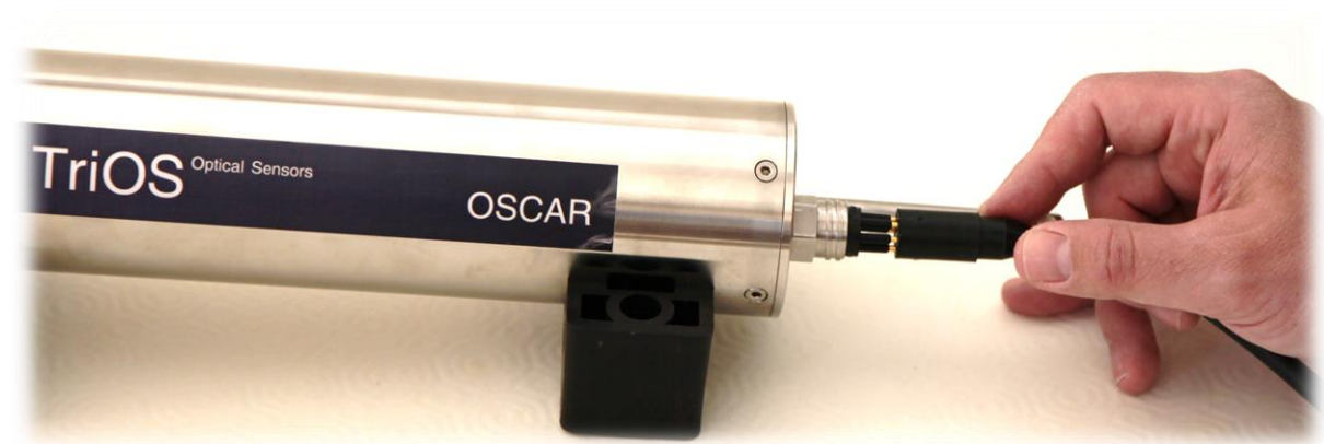
Fig. 3. Carefully aligning the pins onto the connector
