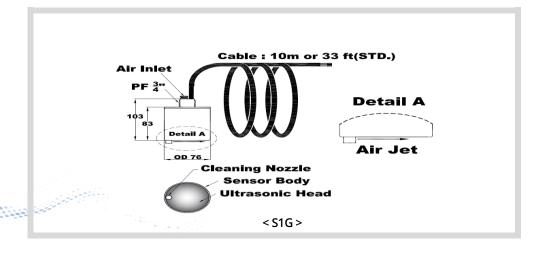
ENV120 is equipped with a cleaning nozzle inside the ultrasonic sensor to automatically clean the sensor surface. Periodical sensor cleaning is recommended as a precaution since floating debris and biological material is in contact with the ultrasonic sensor. When using the air-line on site, a sensor cleaning device equipped with a solenoid valve is supplied as an option.
