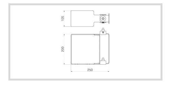
Controller and Cleaning device mounting kit is used for installation of controller or cleaning device. Hand-rail type of controller and cleaning device mounting kit are provided to make installation and maintenance easier.
