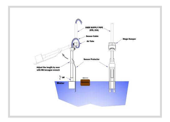
Sensor mounting kit is designed to use hand-rail or ground installation. This SMK helps easier sensor maintenance work.
