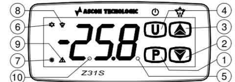
**1 - Key P** : Used for setting the Set point (press and release) and for programming the function parameters (hold pressed for 5 sec.). In programming mode is used to enter in parameters edit mode and confirm the values.
