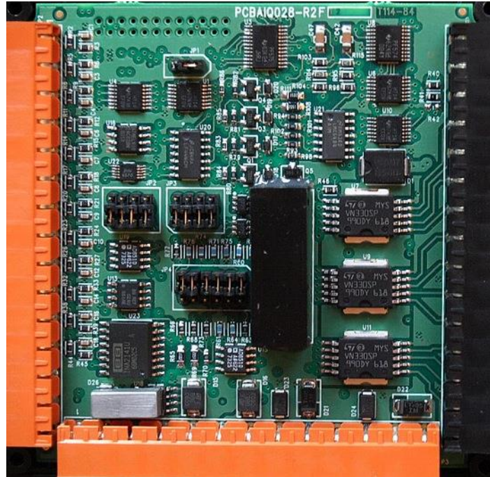
Figure 10.2 – XL+ I/O Cover Removed (sample I/O board)
