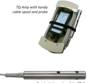
Conductivity probe of the TQ-S
