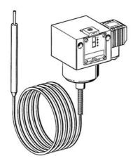
The sensor cartridge at the end of the capillary tube is the actual active (temperature-sensitive) part of the sensor. Changes in temperature on the capillary tube have no effect on the switching point. Pressuretight installation of the sensor in pressure vessels of all kinds is possible with the aid of immersion tubes. (Immersion tubes see page 34).
