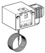
Frost protection thermostats reliably monitor the temperature in hot water-heated air heaters. If the temperature falls below the set value, the thermostat switches off. A visual or audible »frost hazar« alarm can be switched on at the same time. A fixed stop on the setting spindle at 3 °C prevents the thermostat from being set below the freezing point due to inexpert adjustment.
