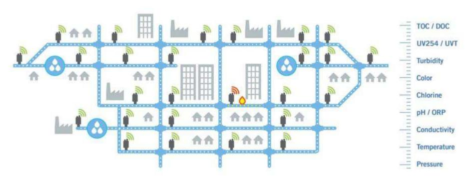
Multiple pipe::scans are the ideal solution to monitor drinking water at any point in the network.
