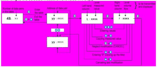
Conditions of correct programming of the data pairs
