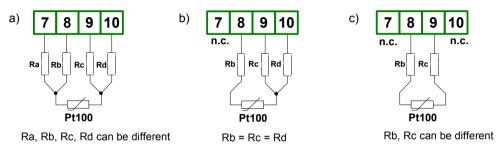
Figure. 4.7. Connection of sensors: a) 4-wires circuit; b) 3-wires circuit; c) 2-wires circuit;
