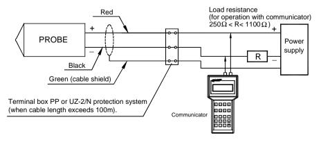
Figure 2. SGE-25.SMART and SGE-25S.SMART probes – connection method
