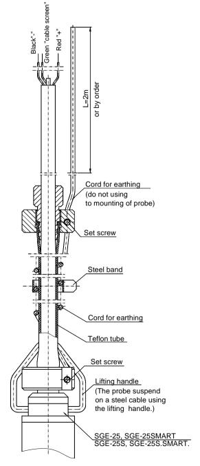
Figure 4. The probe in Ex-version with a cable with an Teflon shield.
