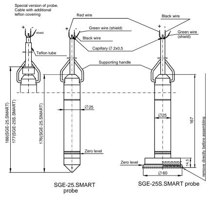
Figure 1 SGE-25.SMART and SGE-25S.SMART probes – dimensions
