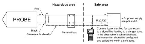
Fig.3. SGE–25.SMART, SGE–25S.SMART, SGE–25C.SMART probes in Ex version – connection method
