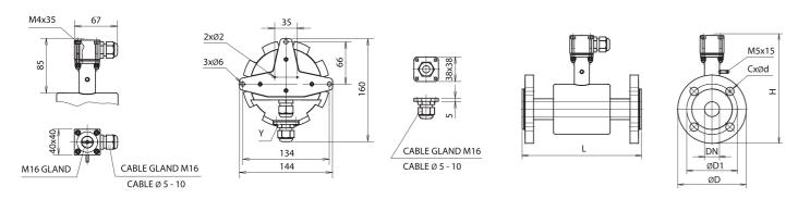
Tolerance of built-in length: DN 10 – DN 150 L±5 mm DN 200 – DN 1000 L±10 mm
