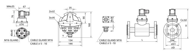
Tolerance of built-in length: DN 10 – DN 150 L±5 mm DN 200 – DN 1000 L±10 mm Standard pressure: DN 10 – DN 50 PN 40 / 150 lbs. DN 65 – DN 150 PN 16 / 150 lbs.
